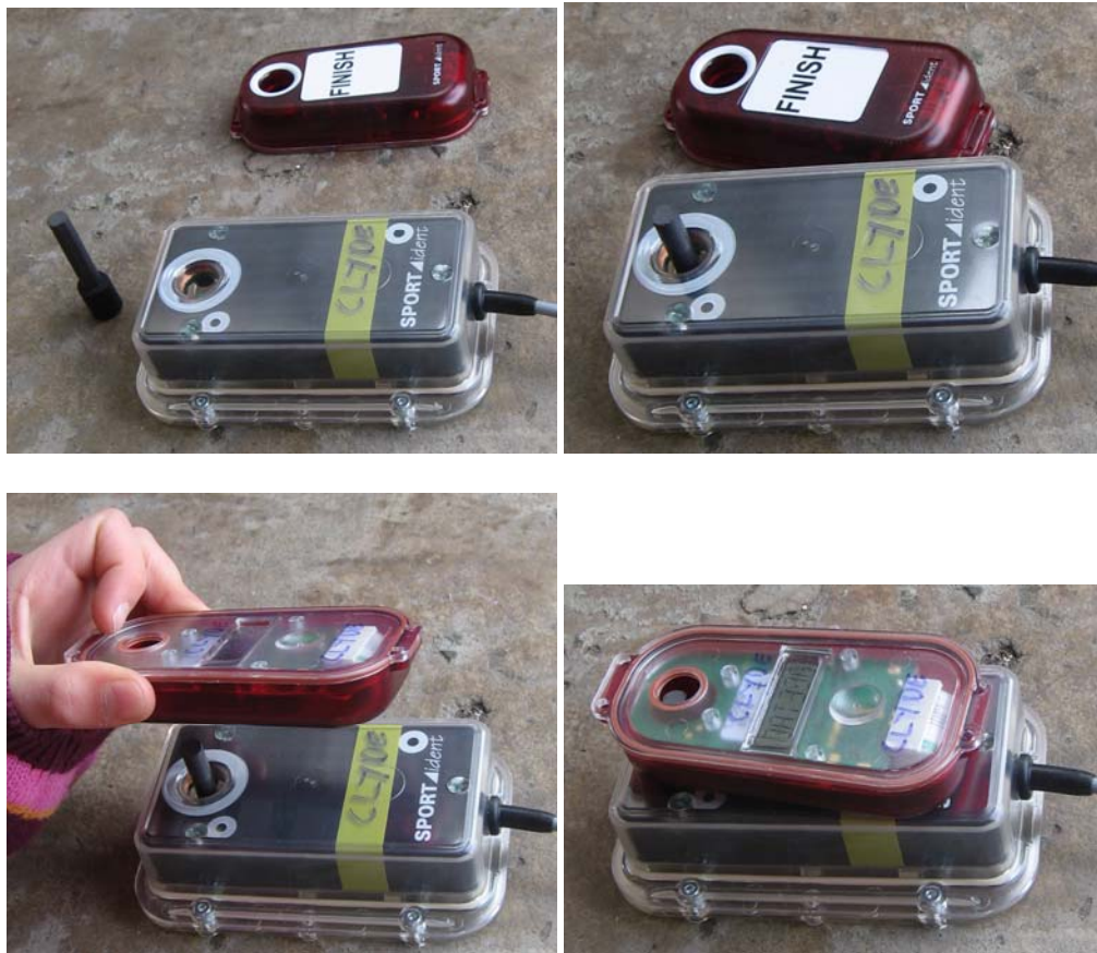
Figure 14 Coupling a unit (start, stop, clear or control) to the DOWNLOAD/MASTER box. You can then read out the unit, renumber it, set the time etc
