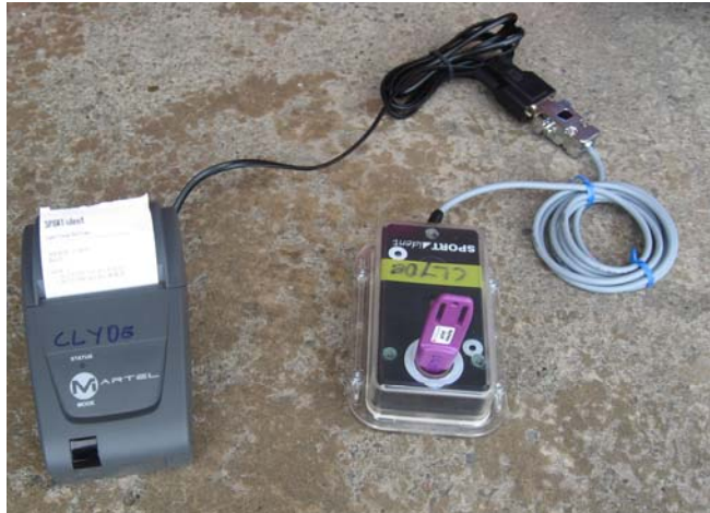
Figure 8 Printing results. Note the "print results" dibber should be used like a normal dibber. Leave it in too long and you will print multiple copies of the results
