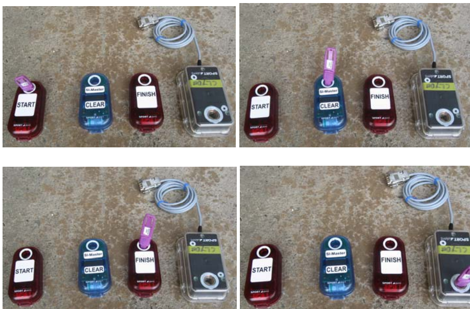
Figure 2 Clearing the START, CLEAR, FINISH and DOWNLOAD/MASTER boxes. The boxes should beep and flash like normal control boxes
