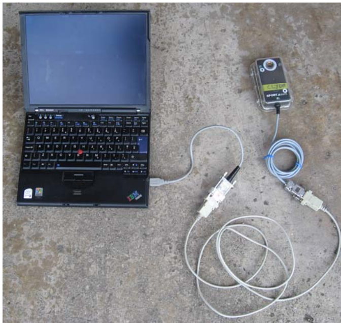
Figure 13 Laptop coupled to DOWNLOAD/MASTER box. Computer needs to have SI config installed
